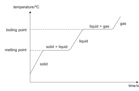
At parts where the graph rises, heat is supplied to the substance to raise its temperature. The graph becomes flat when the substance undergoes a change in state. The graph remains flat as heat is taken in to overcome the interactions between the particles.
