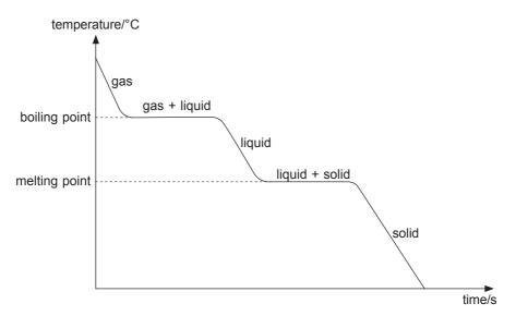
At parts where the graph falls, heat is given out from the substance to the surroundings and its temperature decreases. The graph becomes flat when the substance undergoes a change in state. The graph remains flat as the particles form bonds, producing heat which is given out to the surroundings.
