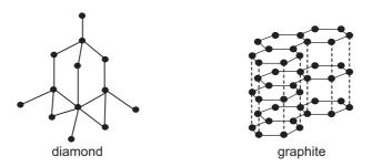
Each atom in diamond is covalently bonded to four other atoms. Due to its rigid structure, diamond is a very hard substance and is used for drill tips or cutting tools.
